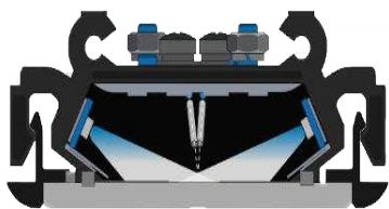
and low power consumption. The 144 tri-color LEDs (42 and 36 inch models) built into the **SingleSensor** never need cleaning and are designed to last the life of the scanner. Colortrac **ClearView** lighting eliminates the effects of shaded areas caused by creases or folds in a document and removes the sensor to sensor differences often seen in older design modular CIS scanners.
