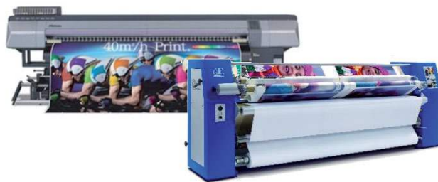
Dye sublimation is a two-step process requiring a specialised textile calender
